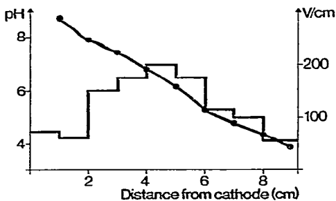
Fig. 4. Apparent pH gradient and field strength in an Agarose-IEF gel with 8 M urea after focusing for 1800 V h.
